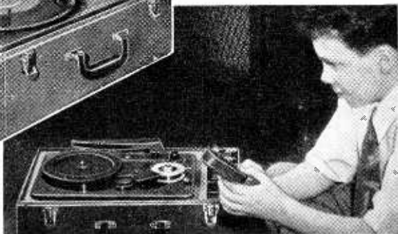
—the U.S.A. Known as the Wireway recorder it weighs only 22½ lb.
